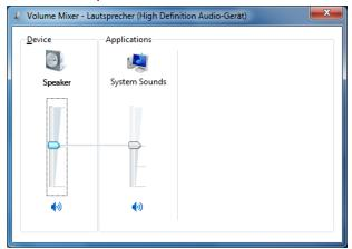
By using the keys Fn + F7 and Fn + F8 you have the possibility to regulate the volume.
