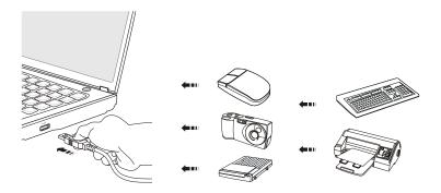
Some USB devices require that you reinstall software drivers when you connect the device to a different USB port than the one originally used. This can be avoided by always using a certain device with the same USB port.
