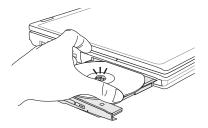
4. Test that the disc is able to turn freely and then push the tray back into the optical drive carefully.
